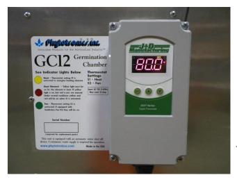
To change the fan activation temperature, Press "SET" 2X from "run mode". OUT2 will be on the top edge of the display and the number will slowly blink. Factory set at 80. The arrow keys are used to raise or lower this number. Once the desired temperature is set then push "SET" once to enter "run mode" for example at 80 the unit will need to reach an internal temperature of over 82 for the fans to come on and if cool enough outside then they will pull it back to 80 before they will turn off.
