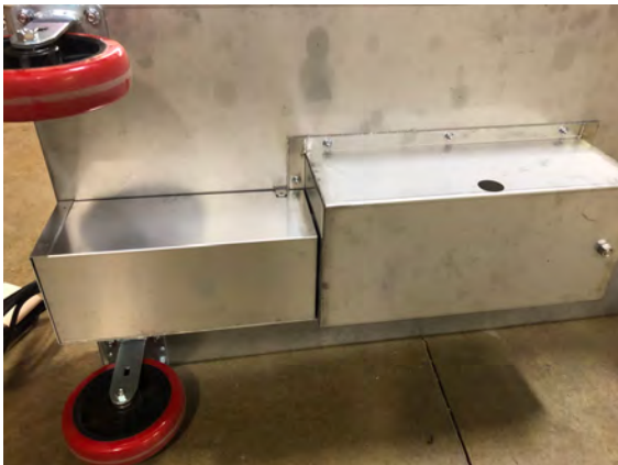
Electrical Box Cover on the left. Water Reservoir on the right with drain plug nut visible.
