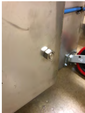
Drain nut outside bottom of water reservoir.
