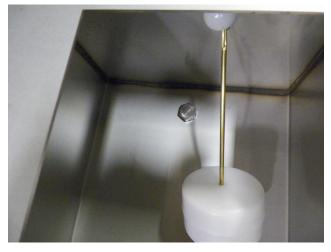
6. Locate the drain nut on the bottom side of the tank.
